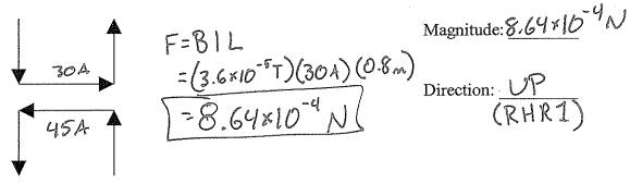
Hint: What is the strength of the magnetic field, caused by the bottom wire, where the top wire is?  $B = \frac{\omega_0 T_B}{2\pi r} = \frac{(4\pi \times 10^{-7})(45A)}{2\pi r} = 3.6 \times 10^{-5} T$
